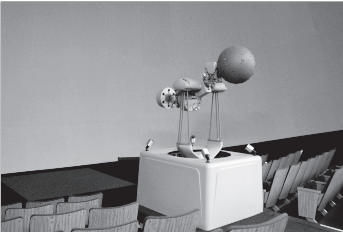
Below: The Spitz 512 projector housed in a 40-foot tilted dome with 90 unidirectional seats
